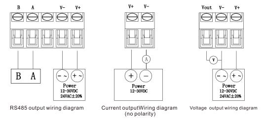
\* When the RS485 type uses AC power supply , it is necessary to use isolated AC power supply , otherwise it may damage related connected devices.
